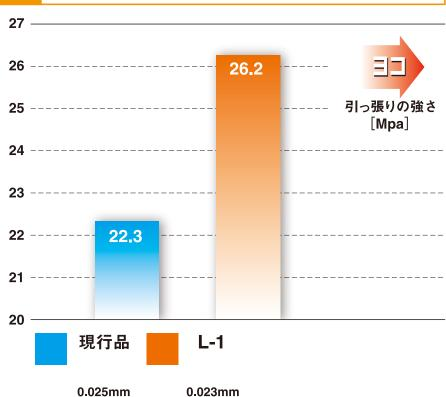
The technology of our company, which had been remarkable improved in recent years, developed the "L-1" the advanced LLDPE film.(linear low-density polyethylen) The most important advantage of "L-1" is its strength. The strength test proved that the 0.023mm L-1 is stronger than the standard 0.025mm LLDPE.
